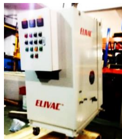
Mobiles Transformator Service System
